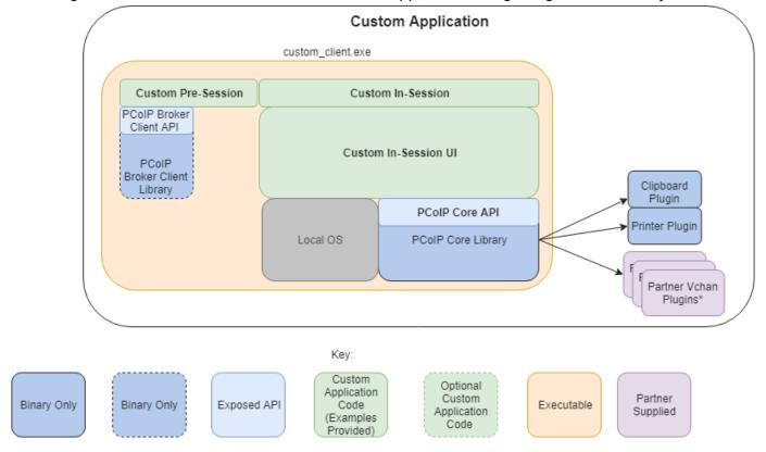
This diagram shows the architecture with a custom application integrating the core library.
