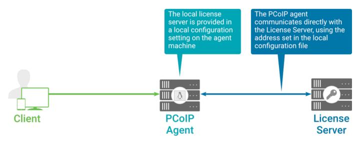
Local license validation using a Remote Workstation Card Agent for Linux and a direct (unbrokered) connection
