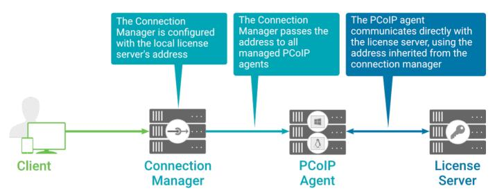
Local license validation using a Remote Workstation Card Agent for Linux and a brokered connection
